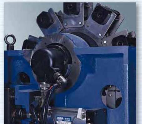
■ ATC magazine activated by servo motor (H500A)
